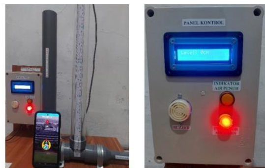
Fig. 9. Test results of the device with a water level of 0 cm
