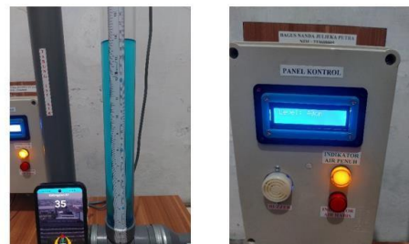
Fig. 10. Test results of the device with a water level of 35 cm
