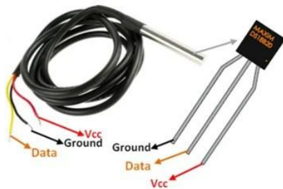
Figure 5 DS18B20 temperature sensor
