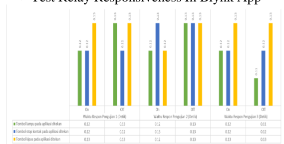
Figure 10. Relay Responsive Test in the Blynk Application
