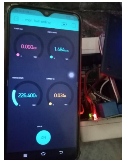
Figure 4.4 relay testing using android O . condition
