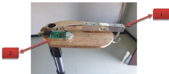
Figure 6. Load cell sensor for measuring weight of infus
