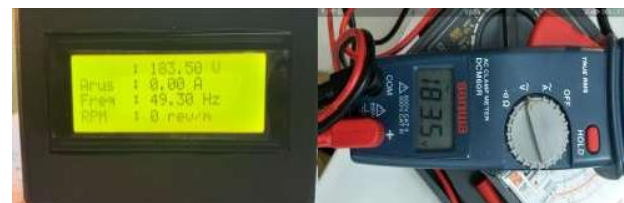
Fig.5 Voltage Sensor Testing on LCD and Avometer
