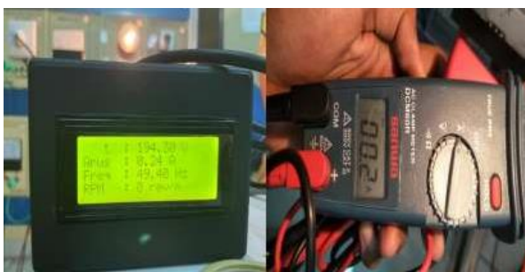
Fig.4 Current Sensor Testing on LCD and Avometer
