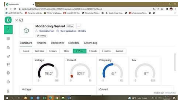
Fig.5 Current Sensor Test on Blynk
