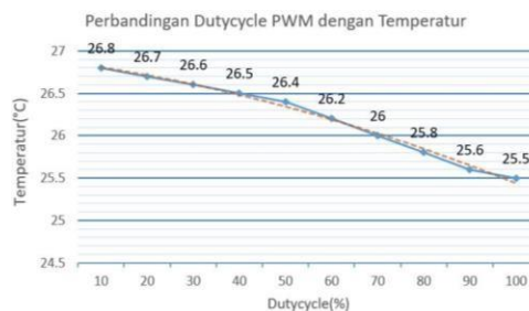
Fig. 12. Comparison Graph of PWM Duty Cycle and Temperature
