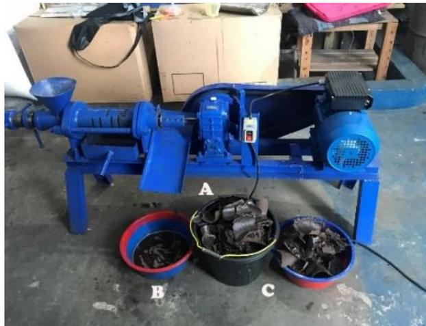
**Gambar 2.** A. Mesin screw press, B. Minyak biji kapuk, C. Residu pengolahan biji kapuk
