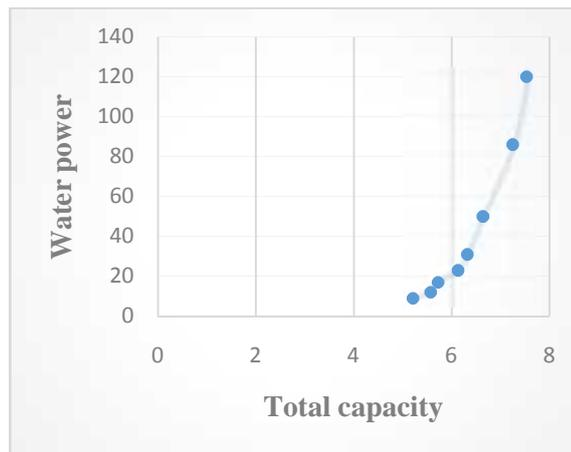
Figure 5: Relationship of water power and total capacity
