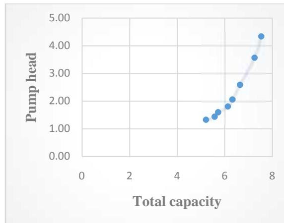
Figure 4: Relationship of pump head and total capacity
