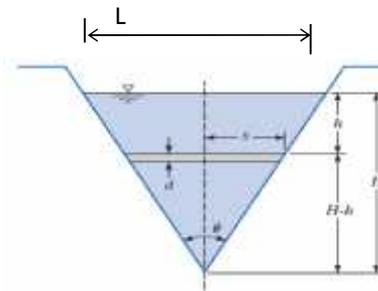
Figure 1: V-Notch Weir
