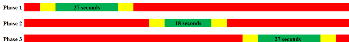
Figure 7. Three-phase traffic light simulation results with a modified Norwegian system
