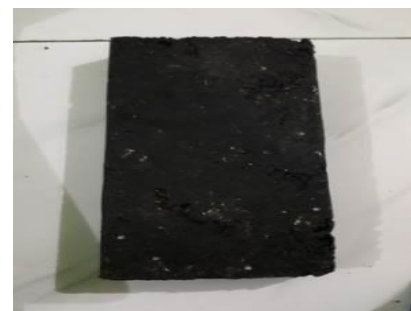
Gambar 3. Paving Block Sampah Plastik
