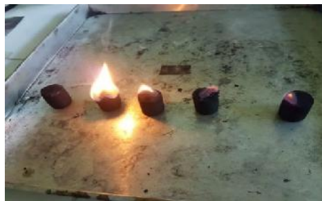
Figure 3. Combustion Rate Test on Biobriquettes
