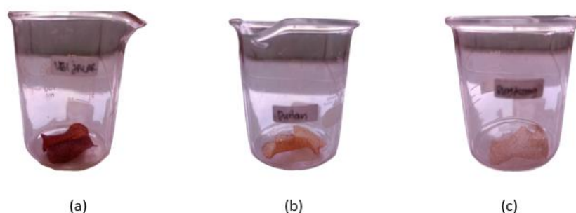
Figure 4. Biodegradable Plastic After Drying (a) Purple Sweet Potato Starch Film, (b) Durian Seed Starch Film, (c) Cassava Starch Film
