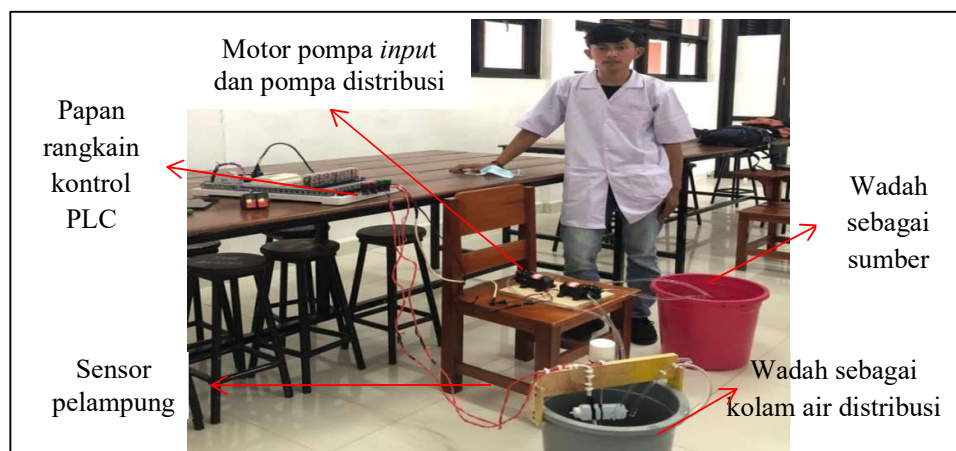
Gambar 5. Skematik prototipe alat kontrol otomatis dinamo water pump PDAM
