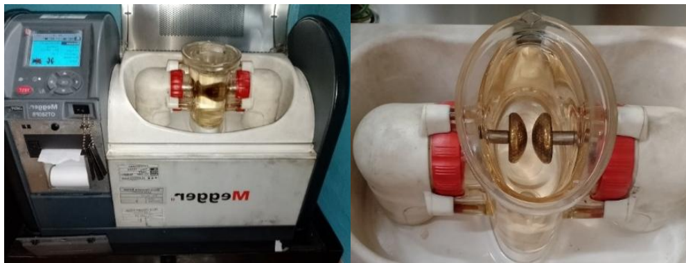
Figure 1. Breakdown Voltage (BDV) Tester
